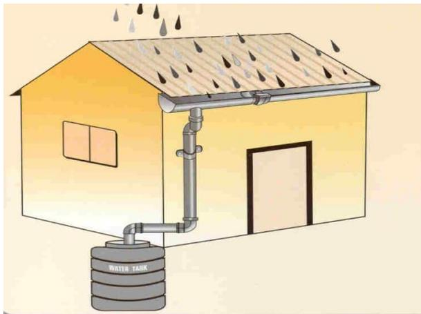
Figure 5: Roof dependent RWH-system (Madhya Pradesh Pollution Control Board , 2013)
