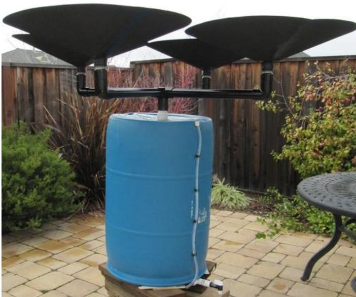
Figure 7: Example of a Rain Saucer design (RainSaucers, 2009)
